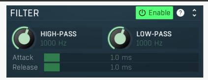
Filter panel controls filter processing. There is a specific set of sequences for filtering as well as for time and volume. Filter sequences control the cut-off frequencies of a variable band-pass filter and here you can set its properties. This processing takes significant amount of CPU, causes phase shift and change of spectrum even in 100% state, therefore it is disabled by default.
