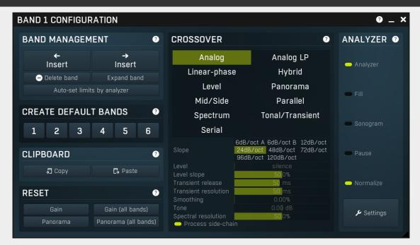
Band menu provides features to control the set of bands and copy & paste band settings (**Band management** section), reset band input gain & panorama (**Band gain & panorama** section), and to select and customize the crossover (**Crossover** section) and analyzer options.
